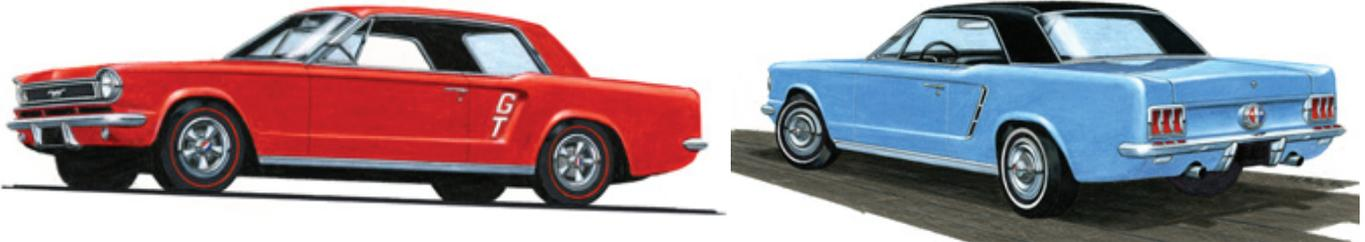
I based this car on the Rambler American 2-door hardtop. By extending the wheelbase and front clip forward of the cowl, chopping the top and blanking out the C-pillars, I came up with a "Mustang" that looks surprisingly like the original.
